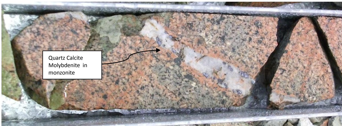
Figure 2 – Quartz-calcite-molybdenite-pyrite-chalcopyrite vein in monzonite in hole TD002 420m, Trundle Park prospect. The one metre interval containing this vein returned 1190ppm Mo within a larger zone of 100m @ 34ppm Mo from 357m b (NQ core).
