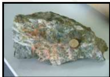
Quartz-K-feldspar-chalcopyrite breccia (>40g/t Au)
