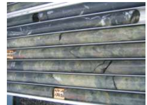
ALRCD001 169-174m epidote altered breccia
